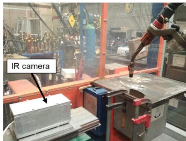
Figure 8-13: Deposition of the WAAM samples.
