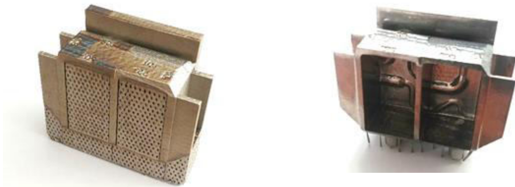
Figure 7-22: Samples 1.4404 (left: as built, right: after hirtisation).
