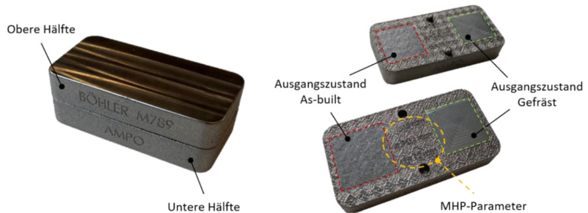
Figure 7-45: Use-case part for MHP treatment of the AMPO M789.
