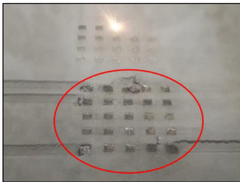
Figure 6-14: Job failure on DMG MORI Lasertec 2nd Gen. using the process parameters from TRUMPF SLM machine for M789 AMPO.
