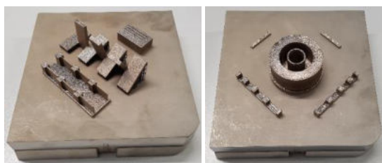
Figure 5-6: Sample geometry for the analysis of resolution, accuracy and surface quality in accordance with ASTM 52902
