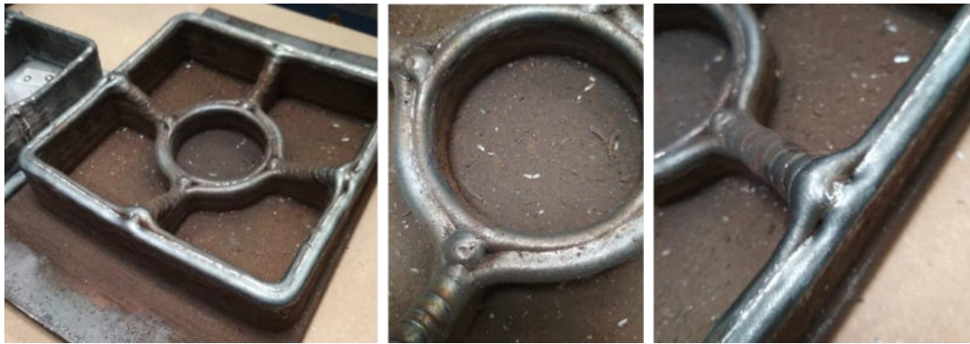
Figure 8-44: Resulting part with unacceptable quality
