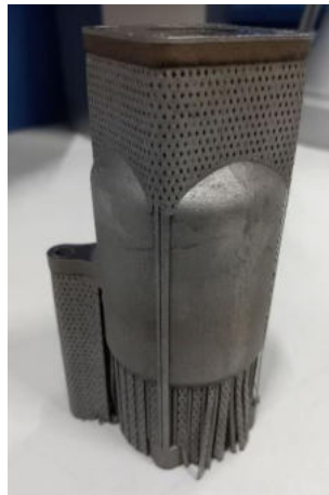
Figure 7-32: Flame arrestor 3D-printed.
