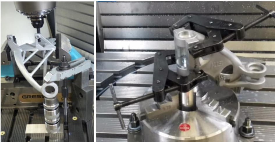
Figure 9-9: Conventional clamping of AM parts for machining [12]
