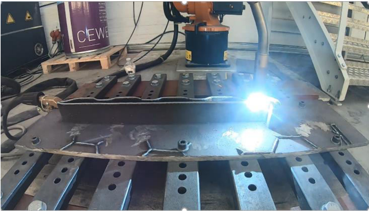
Figure 8-39: Deposition of bridge prototype
