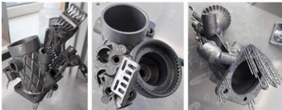
Figure 7-29: Injector Housing after hirtisation.
