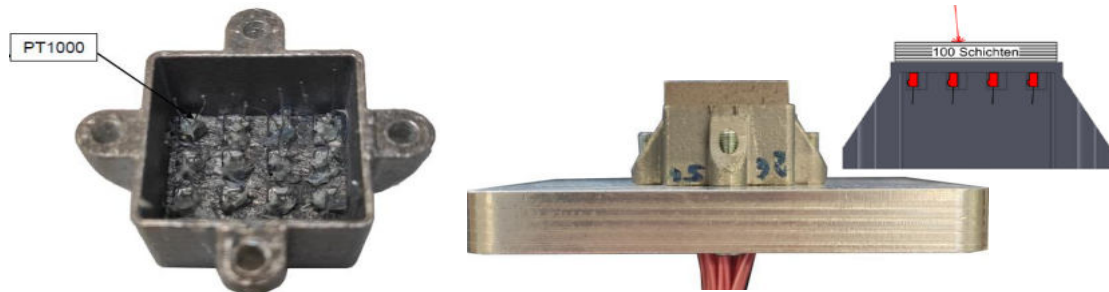
Figure 6-3: Sensory part of the developed DAQ chain [3].
