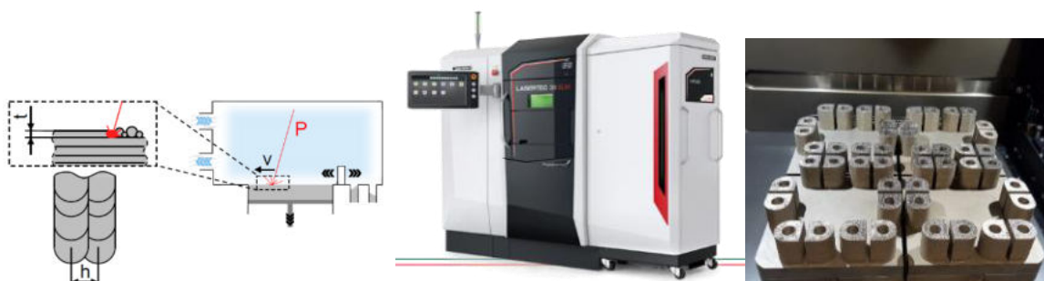
Figure 5-4: explanation of main LBPF influencing parameters (left), used LPBF machine (middle) and example of the build job (right).
