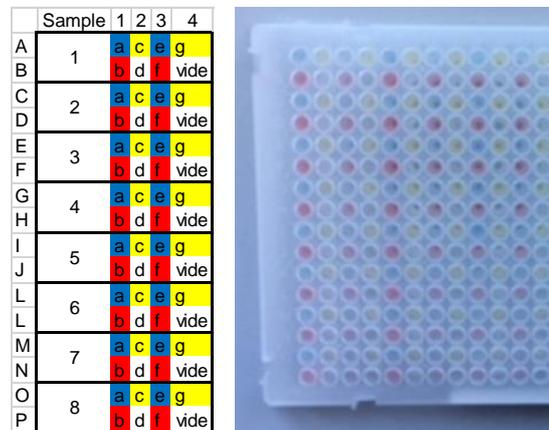
Figure 11. The programmed layout is shown on the left and the Microlab Star<sup>let</sup> pipetting on the right.
