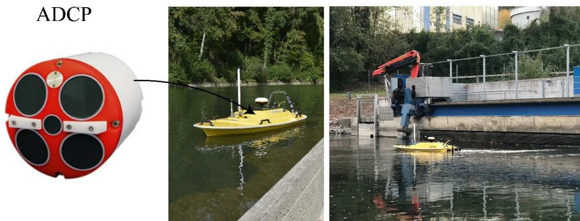
Figure 6: Flow velocity measurements at HPP Schiffmühle using Acoustic Doppler Velocity Profiler (ADCP) with remote controlled boat (ADCP photo: courtesy of Teledyne Marine, USA).
