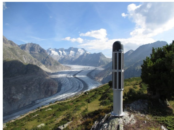
Fig. 1 GNSS monitoring station MOO1 at the “Moosfluh” slope instability in the vicinity of the Great Aletsch Glacier.
