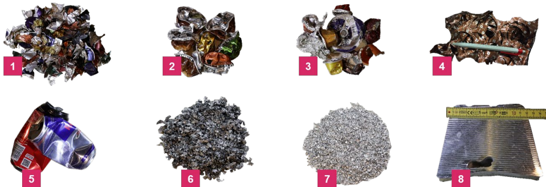
Figure 2.1: Visual aspect of the aluminium samples as obtained from the partners (Sample 1 to 8), before treatment.
