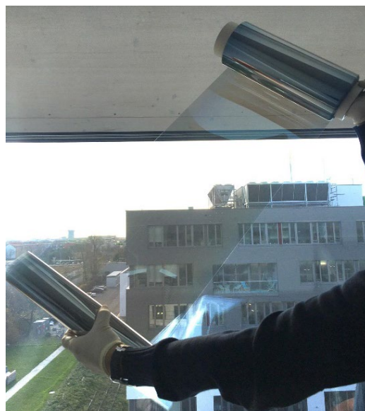
Figure 9. Photo of a 300 mm-wide roll of TNO/Ag/TNO DMD, sputtered according to the developed recipe.
