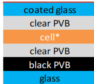
Figure 8: Scheme of coloured BIPV modules designed in the frame of the project.
