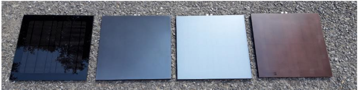
Figure 11: Image of the prototype modules produced by ertex-solar (40 x 40cm) with (from left to right): clear, inkjet printed (grey), screen-printed (grey) and sol-gel sprayed (terracotta) front glass.
