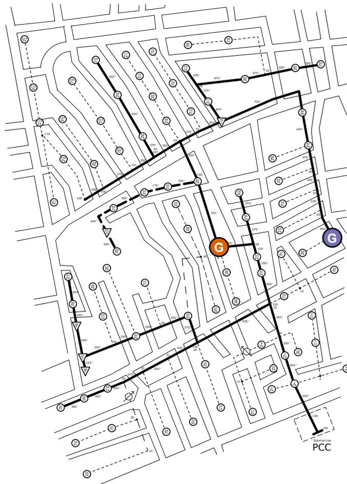
**Figure 9:** The 56-bus feeder proposed as a testbed for the “Optimal generation curtailment in power distribution grids” scenario.
