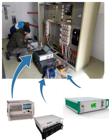
Figure 43 Line impedance measured at a transformer substation in the Alps with 3 different impedance analysers
