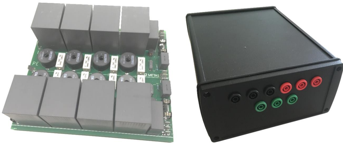
Figure 9: Static line reference impedance additional network PCB (left) and packaged (right)
