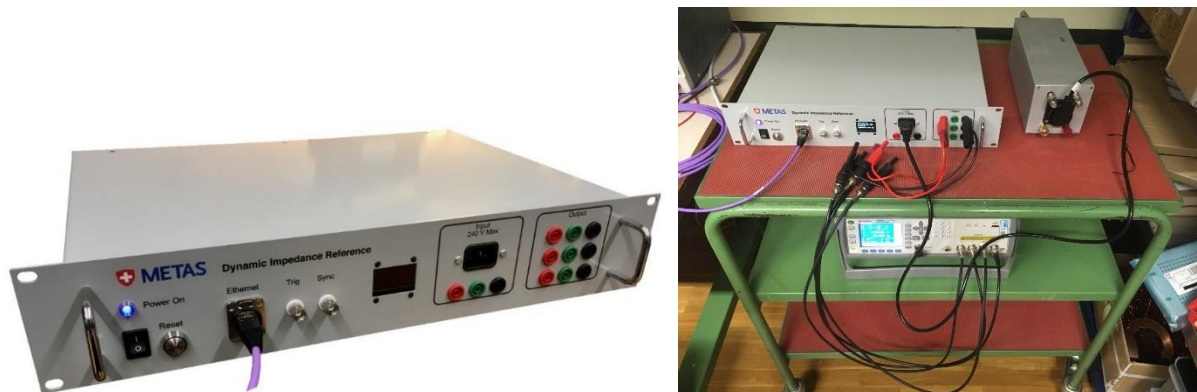
Figure 11: Programmable line impedance reference (left) and automated characterization setup (right)
