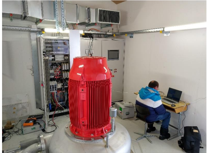
Figure 42: Grid impedance and power quality measurement at the RE installation in the Alps (grid configuration on the left)
