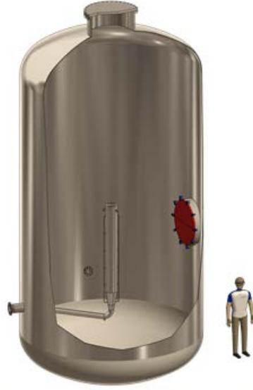
Figure 1.1: Drywell of the experimental PANDA facility with the bent steam injection tube inside.
