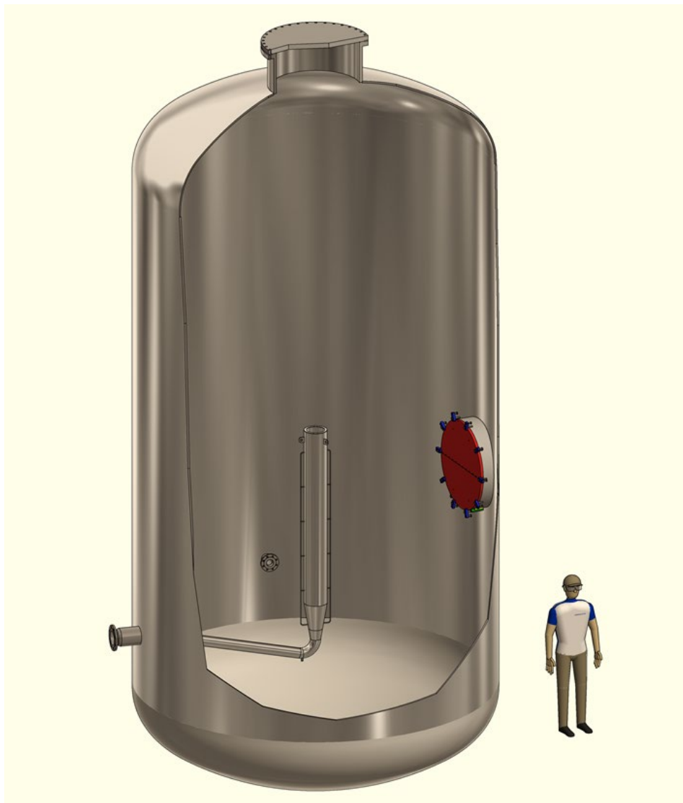
Figure 5.1: Rendering of PANDA Vessel 1 and the injection line.
