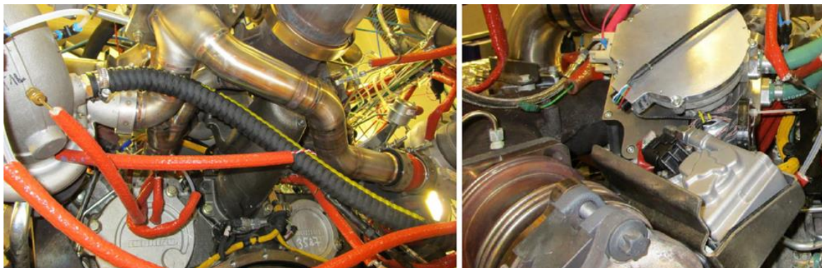
Figure 24: E-charger integrated on the engine with compact piping
