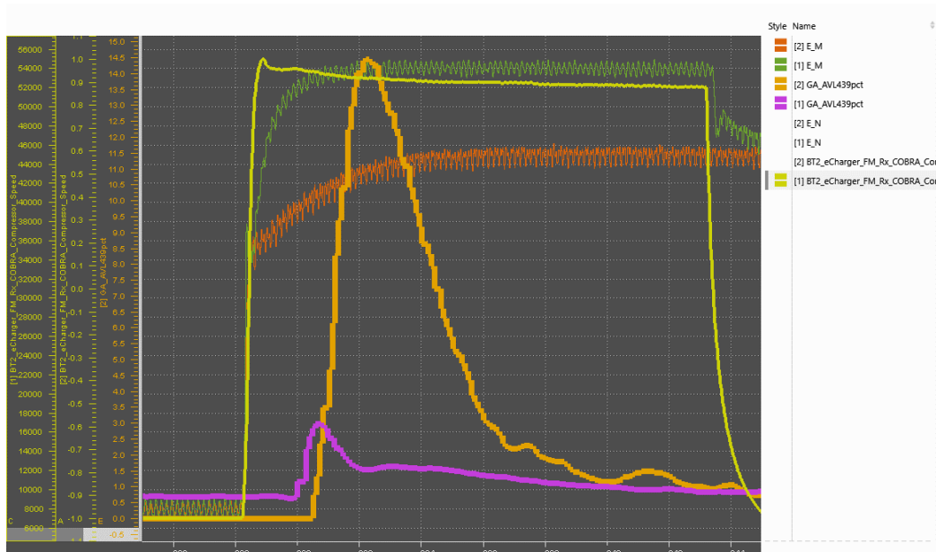
Figure 16: Impact of the e-charger on the exhaust gas smoke: reference (brown); e-charger (pink)
