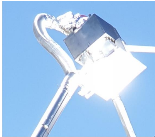
Figure 3.3. The picture of the integrated photo-electrochemical reactor mounted at the focal spot of the parabolic dish concentrator is shown in operation.
