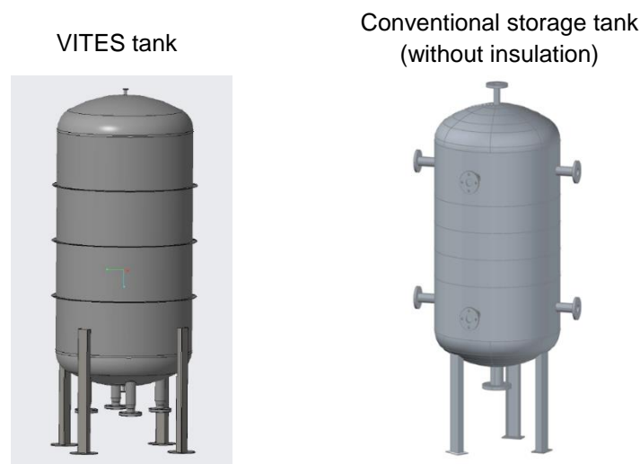
Figure 11 Simplified representation of 1 m 3 VITES and a one-to-one comparable conventional tank (without insulation)
