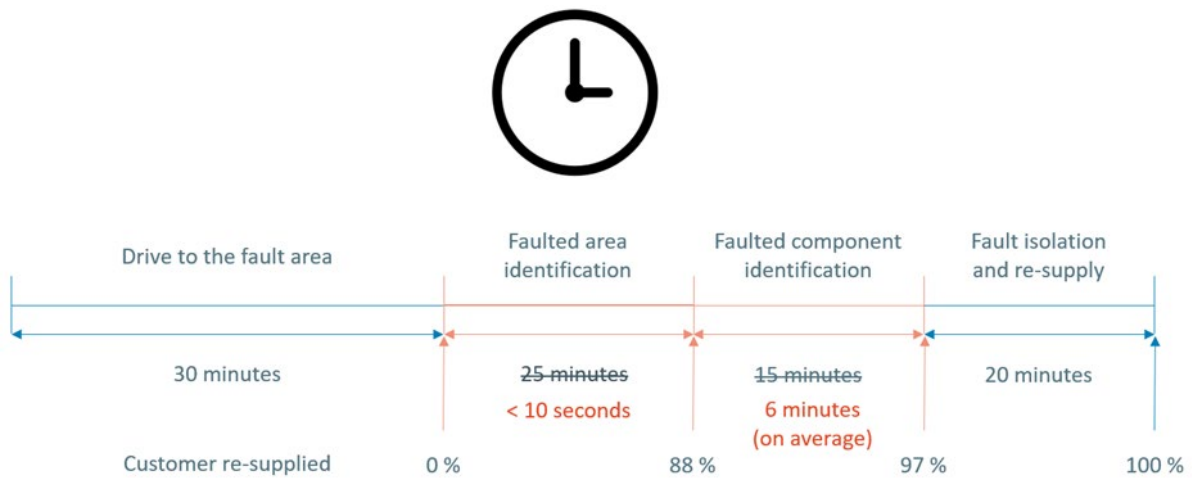
Figure 36: Typical fault location process in BKW distribution grid with average durations of each fault location step
