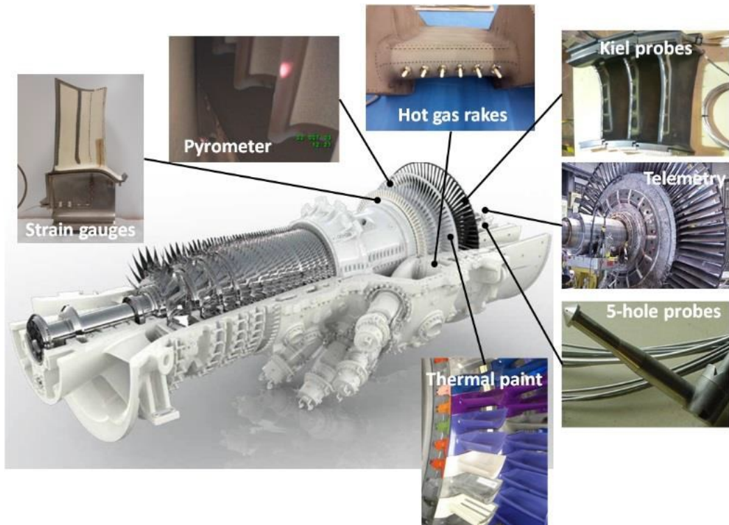
Figure 41: GT36 test turbine and associated instrumentation.
