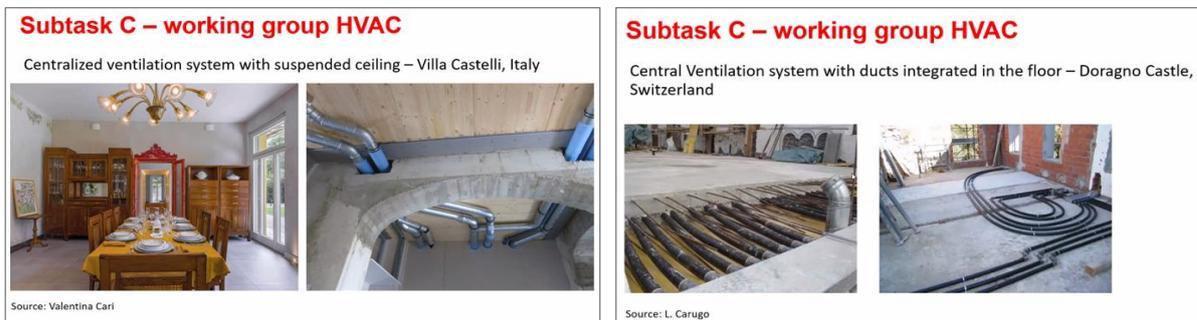
Figure 16. Examples of retrofit solutions documented by the working group HVAC.
