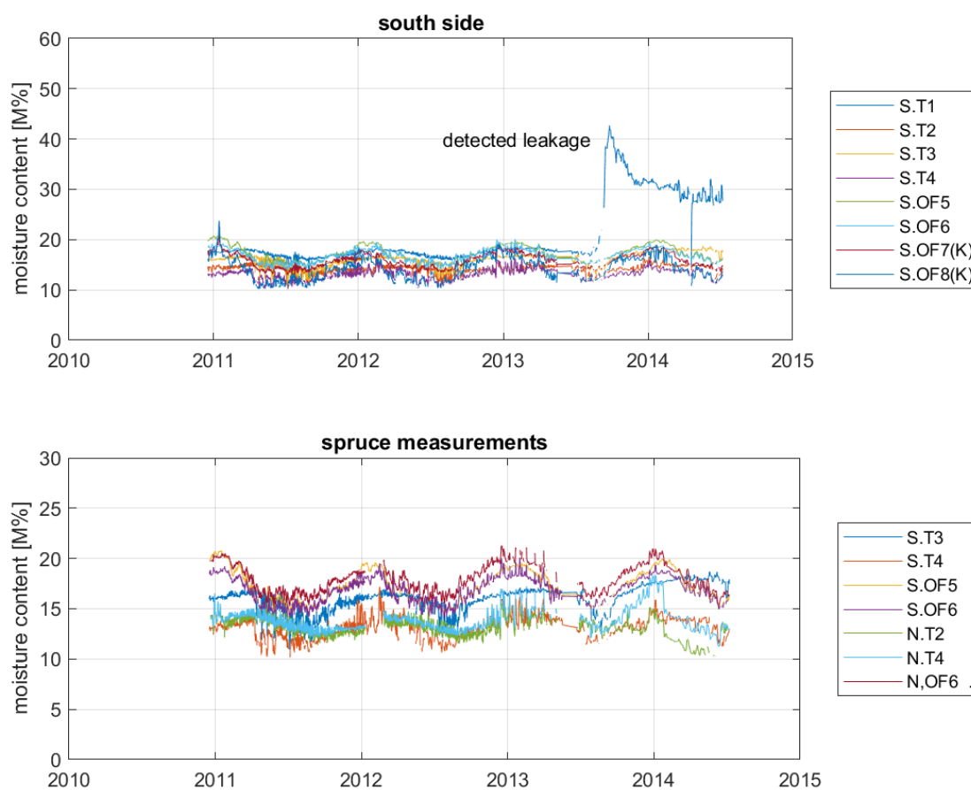
Figure 35: A summary of the moisture content measurements made on the Obermatt bridge where a leakage could clearly be detected thanks to the installed monitoring system.
