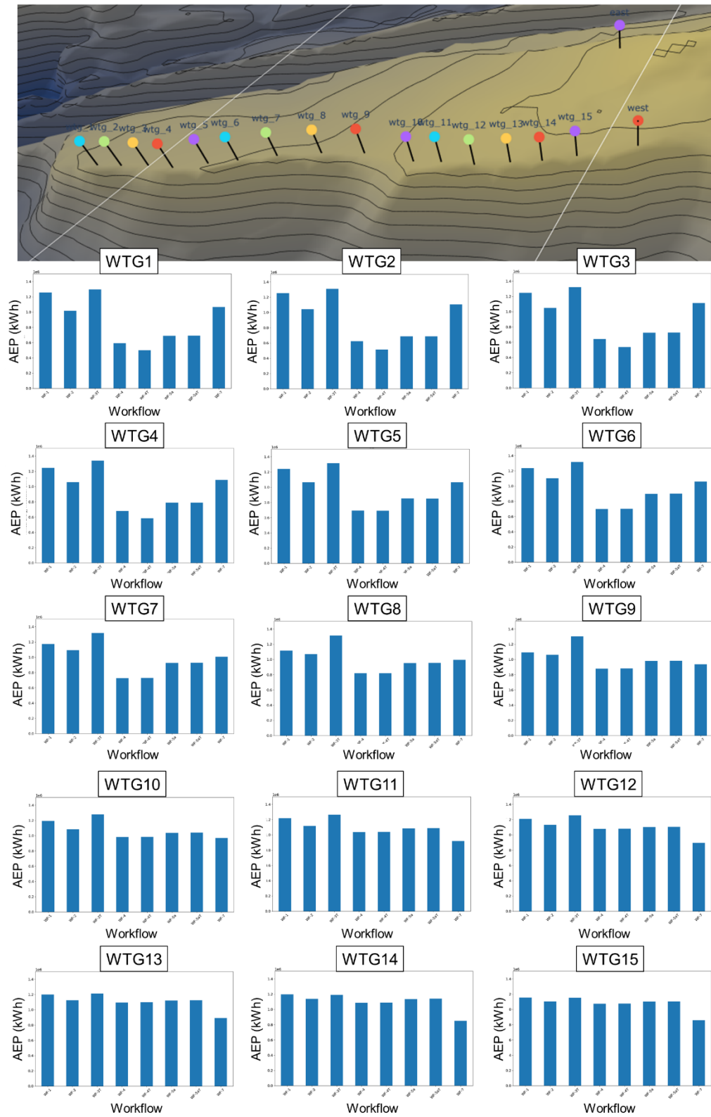
Figure 42. AEP for each Enercon wind turbine WTG1-15 for each workflow (each time from left to right: Theoretical, WF-1, WF-2, WF-3T, WF-4T, WF-5aT, WF-6, WF-7).
