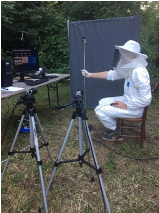
Figure 7: Video tracking system setup in the field. Wild mosquitoes approaching the volunteer are tracked by two cameras placed on tripods and tracked against the dark background. As the handle in the arm-in-cage test, the pole serves to stabilise the exposed arm of the experimenter. Except for the forearm, the person was protected from mosquito bites with a bee keeper's hat, an overall and latex gloves through which mosquitoes cannot bite.
