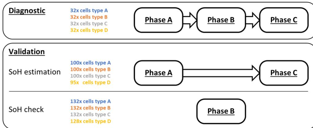
Figure 5 - Combination of the blocks given in Figure 5 to make the testing protocols for diagnostic and validation parts of testing methodology. The arrow entering Phase C implies a voltage regulation phase to reach nominal voltage.
