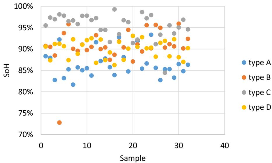
Figure 7 – Measured SoH under diagnostic test - control group – 32 sample for each technology: MJ1 (type A), VC7 (type B), GA (type C) and NC1 (type D).
