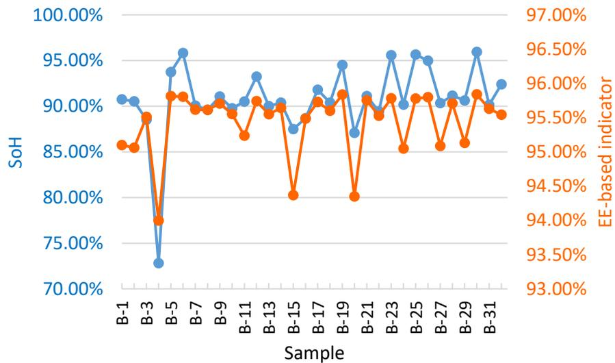
Figure 9 – assessed variables trends at nominal voltage for cell type B (VC7)
