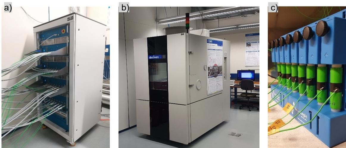
Figure 2 – Overview of equipment and cells in the Energy System laboratory at CSEM. a) Battery tester; b) Thermostatic chamber; c) Cells under testing inside the climatic chamber.
