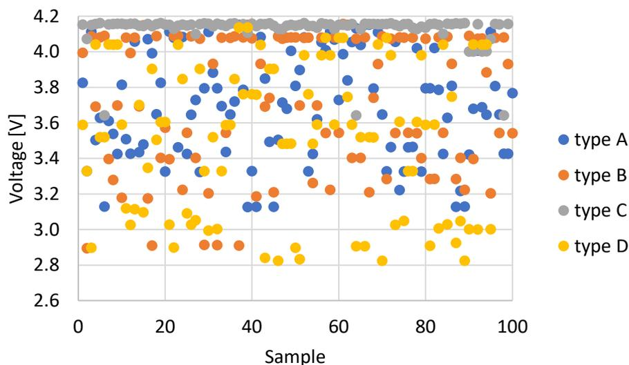
Figure 10 – Initial voltage of the cells under validation test - experimental group – 100 sample for each technology: MJ1 (type A), VC7 (type B), GA (type C) and 95 cells of NC1 (type D).
