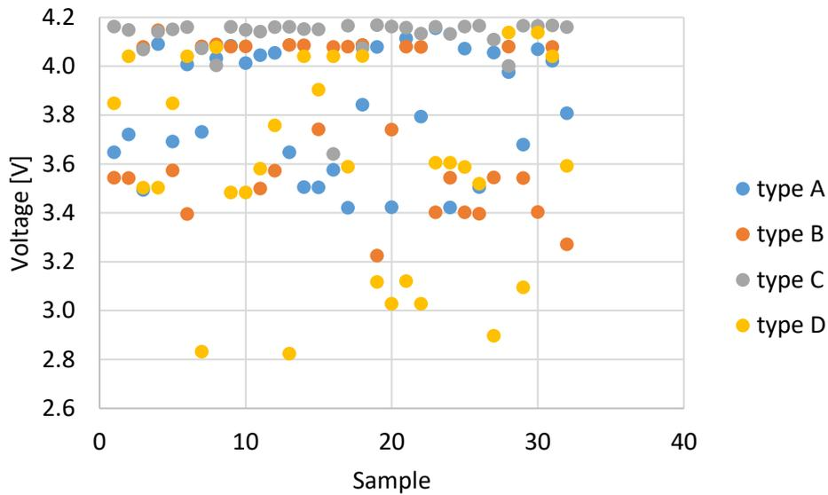
Figure 6 – Initial voltage of the cells under diagnostic test - control group – 32 sample for each technology: MJ1 (type A), VC7 (type B), GA (type C) and NC1 (type D).
