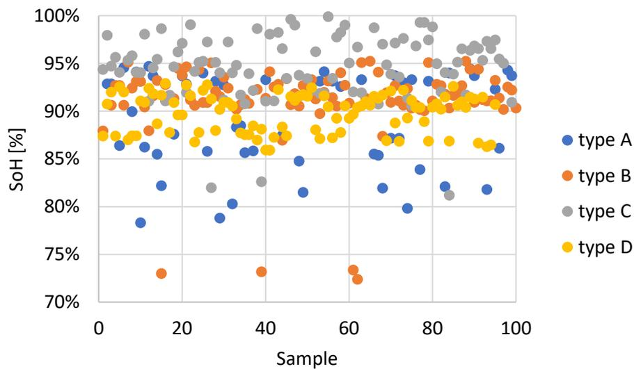
Figure 11 – Measured SoH under validation test - experimental group -: 54 cells of MJ1 (type A), 96 cells of VC7 (type B), 97 cells of GA (type C), and 95 cells of NC1 (type D).
