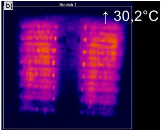
Figure 3 – Overview of equipment and cells at Libattion facilities. a) Battery tester; b) Image taken with thermo-camera to check the temperature of the cells. All the tests are performed at ambient temperature.
