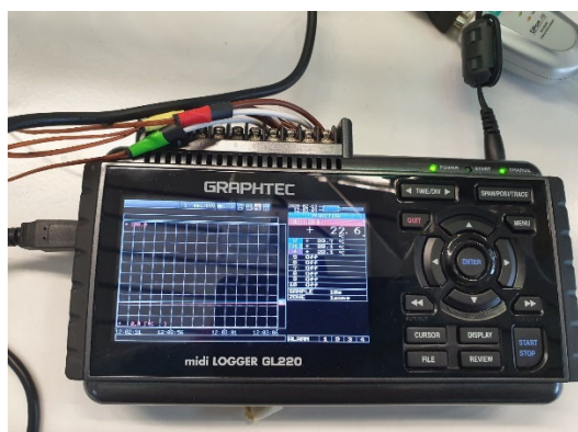
Figure 15: Logger used to monitor and record the reaction temperature during the experiments.
