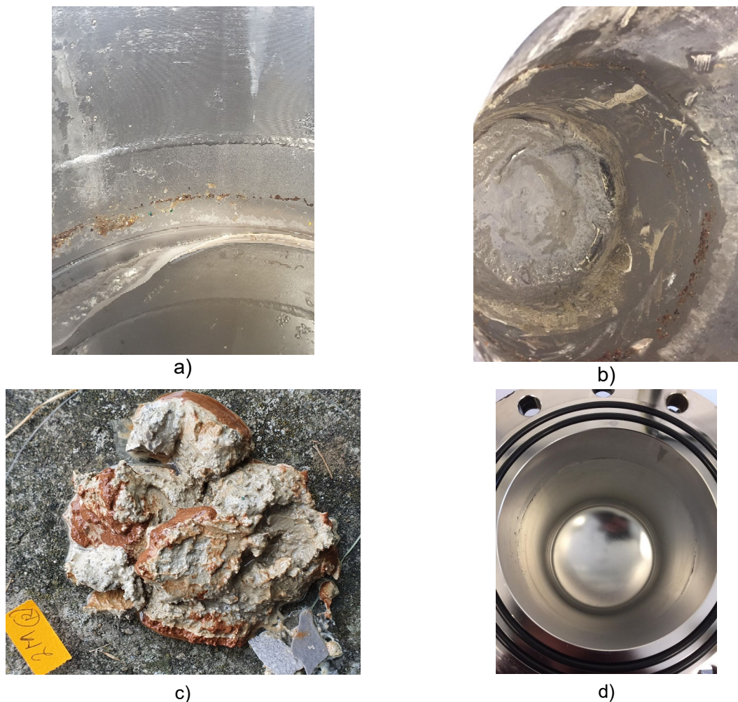
Figure 44: Visual inspection of the converter vessel after the 2 M NaOH experiments, a) upper part with liquid phase, b) lower part with solid phase, c) solid reaction products removed from the converter, d) converter vessel after cleaning.
