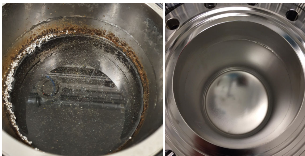
Figure 34: Solid and liquid products from the reaction of 0.5 kg Al grit with the 6 M NaOH solution (left) and vessel after cleaning (right) [14].
