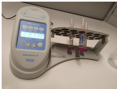
Figure 22: The system used to homogenise the three samples.
