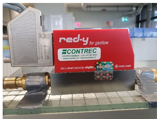
Figure 16: Gas flow meter used for indicating when the reaction has stopped, i.e. when no more hydrogen is produced.
