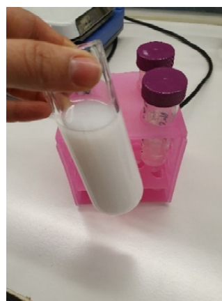
Figure 20: Precipitation of \text{Al}^{3+} occurs when the pH of a saturated solution decreases from 14+ to 12.
