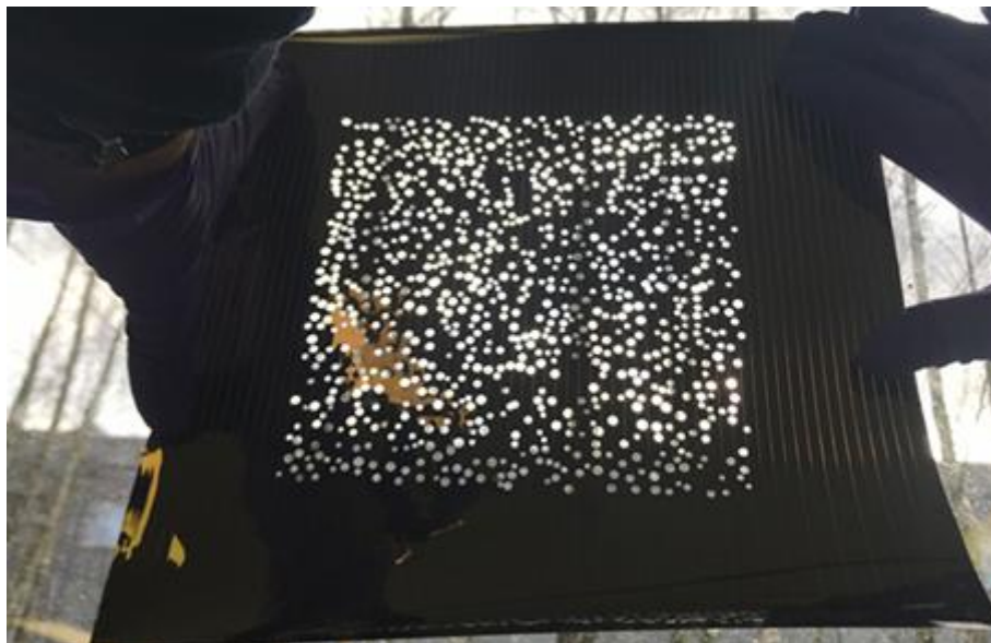
Figure 19: Test sample with approx. 20% transparency by TNO
