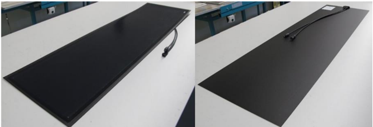
Figure 12: 2x1 reference module using black anodized Al BS. Left is front, right is back side.
