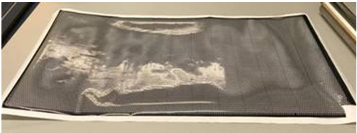
Figure 25: Translucent submodules, showing some bending due to modified residual stress after laser patterning. This requires TNO to laminate already partly the modules before shipping back to Flisom for proper handling and characterization.
