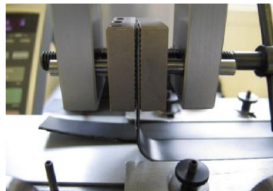
Figure 5: Adhesion measurement with Pull Force Tool
