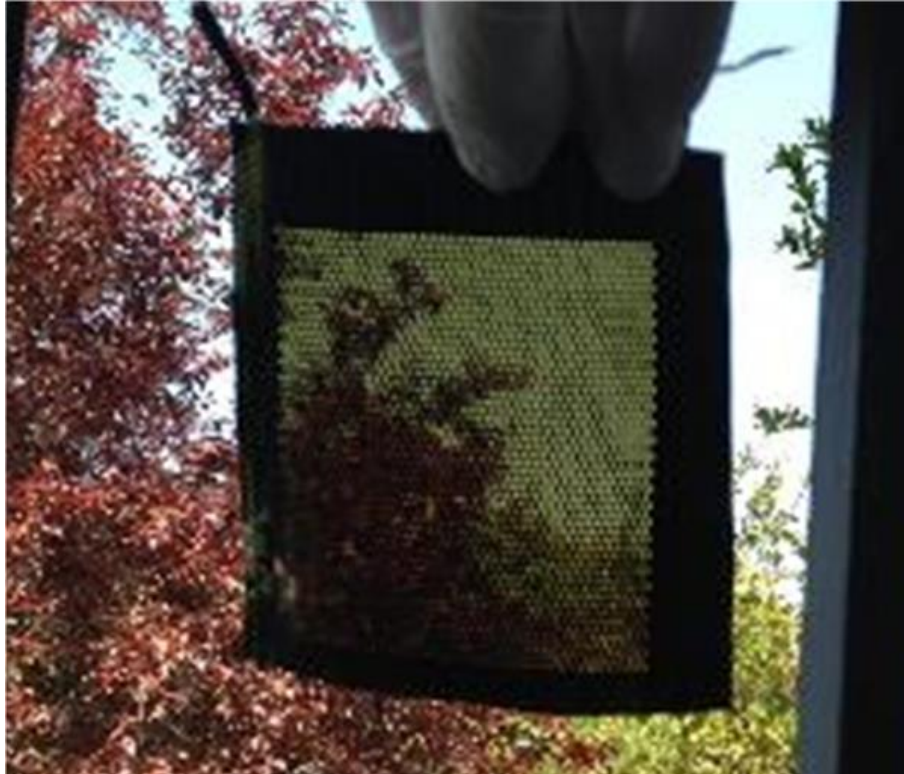
Figure 15 Test sample of laser process by Sunpartner
