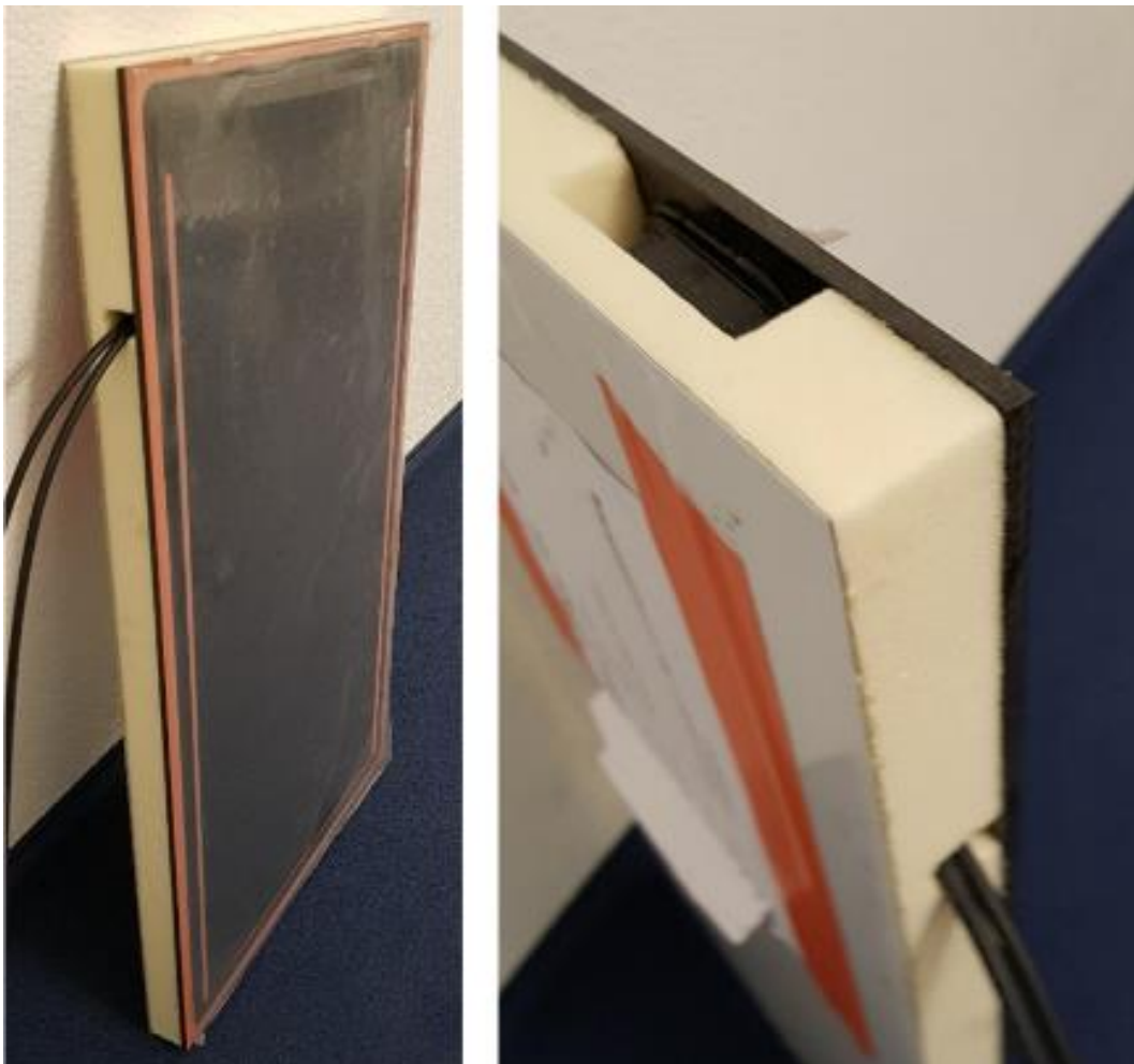
Figure 13: View of a finished sandwich panel based on composite material BS
