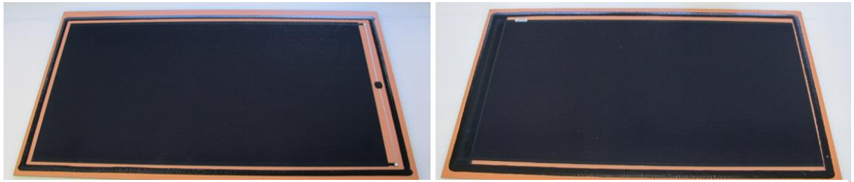
Figure 9: Two 1x1 modules using wooden-composite BS with ES. On the right side the cross contact is covered for aesthetic reasons.
