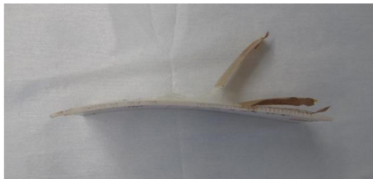
Figure 6 Sample after 6 weeks of DH shows strong unacceptable bend
