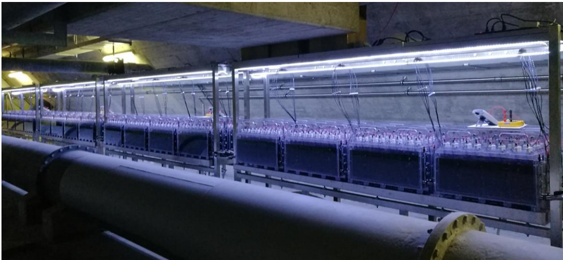
Figure 4: 1000-L MFC with 64 reactor units assembled on 4 carts as stacks. Water and wastewater were introduced from one side (right), passing through 16 MFC-units before reaching the outlet at the other side of the system (outer left). Air flow tubes were branched to the cathodic compartment of each cell. Resistance box and multimeter were connected for electrical parameters determination.
