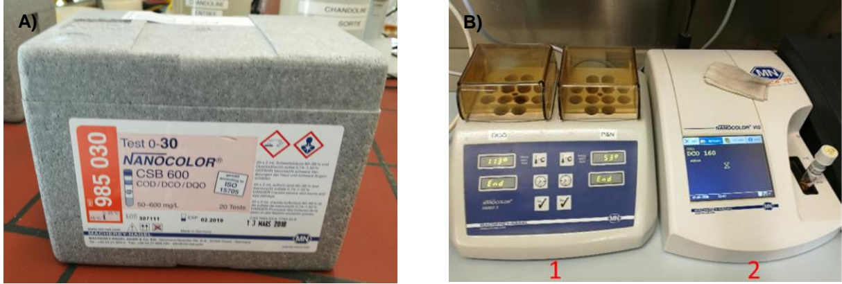
Figure 9: A) Nanocolor® kit employed for COD determination. B) Heating block (1) and photometer (2) used during the COD measurement procedure.
