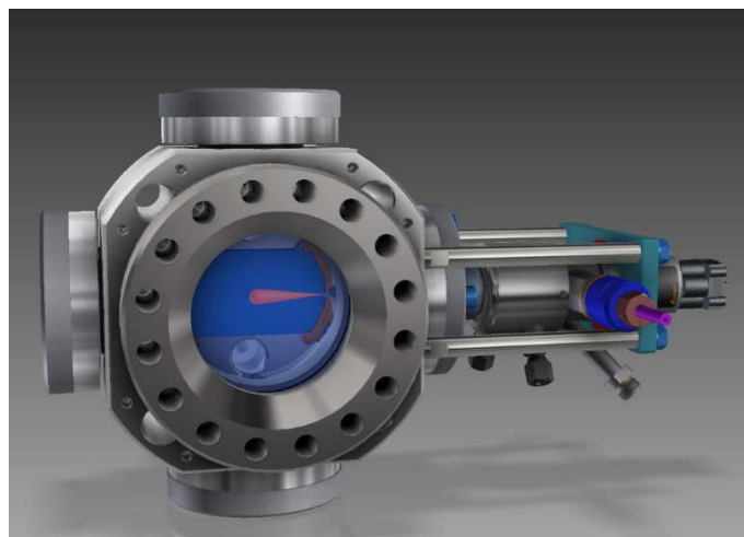
Figure 8. Constant volume cell with the injector mounted on the side.
