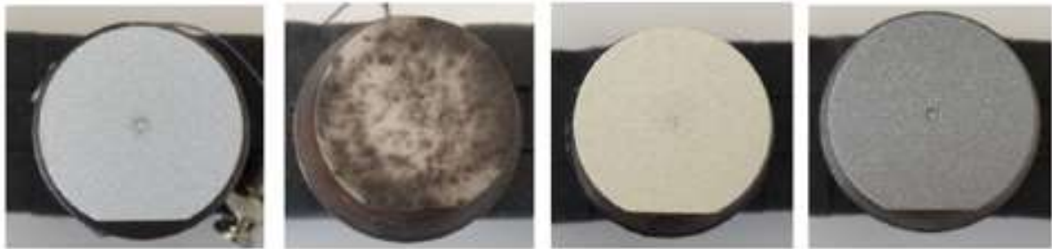
Figure 4. Planned coating materials to be studied: porous aluminium (left), zirconia + sealer (second left), zirconia (second right), zirconia + aluminium (right)
