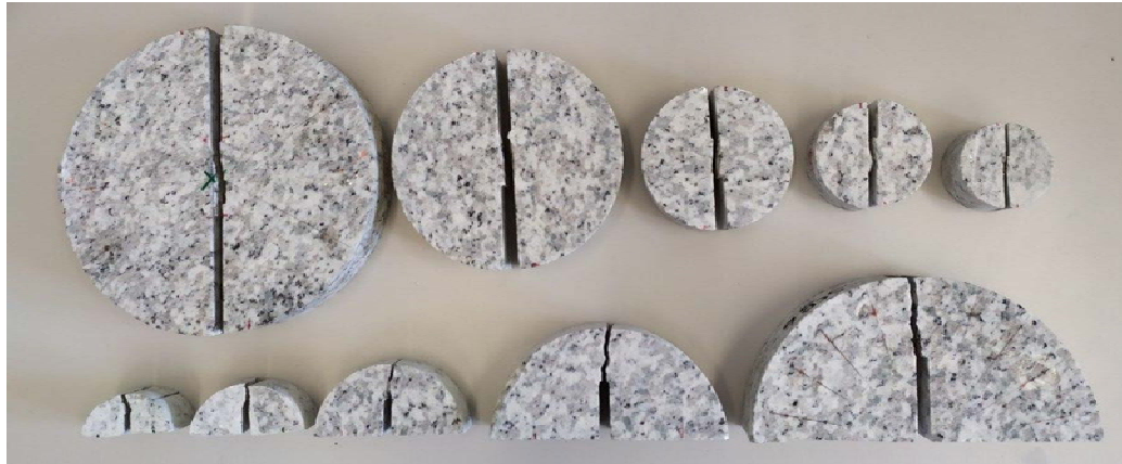
Fig. 5. Fractured DNBD and SCB Bedretto specimens in different sizes.
