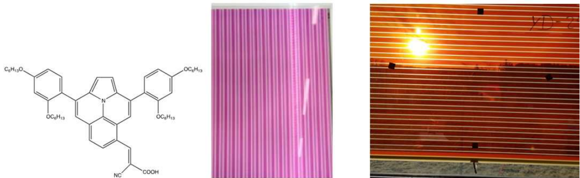
Figure 8: (Left) Structure of the salmon-coloured JD-25 dye developed by LPI_EPFL, JD-25 that has been designed and fabricated for application in the solar sharing project. (centre) Photograph of a DSC panel incorporating the new dye without electrolyte. (right) DSC panel with JD 25 DYE and Livion 14 electrolyte
