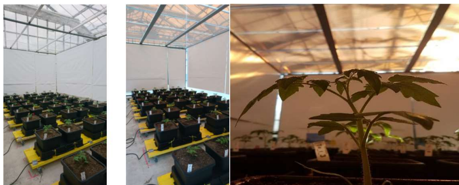
Figure 5: Left: 15 m 2 control module with a glass roof. Centre: 15 m 2 module with red DSCs. Right: Young tomato plants growing under DSC filtered light in the module.
