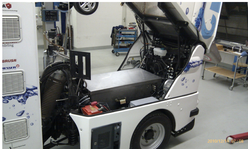
Picture 1: FC box of the hy.muve project vehicle
