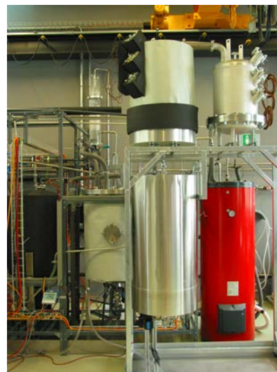
Fig. 22 Picture of the laboratory prototype with the second heat pump and the additional high concentration storage vessel.
