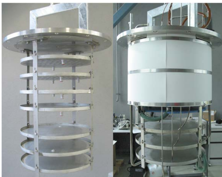
Fig. 15 Initial heat / mass exchanger assembly of the hot and cold exchangers in one vessel. The right picture shows the insulation measures taken.
