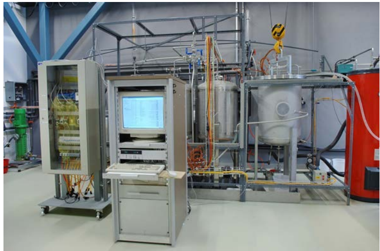
Fig. 14 Laboratory setup of the single stage NaOH sorption storage.
