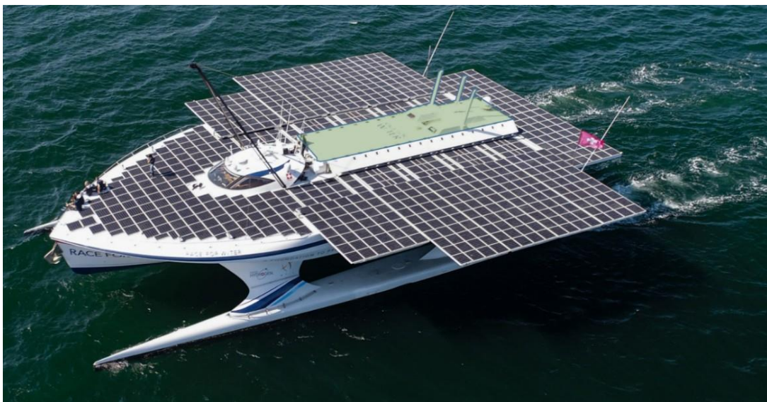
Figure 11: Integrated hydrogen container (highlighted in green)
