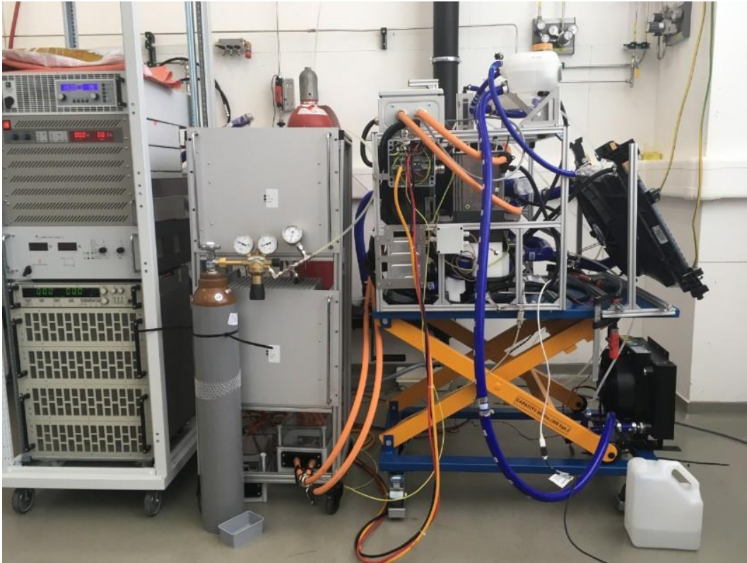
Figure 30: Experimental set-up for the FCS01 for Factory Acceptance Test (FAT)
