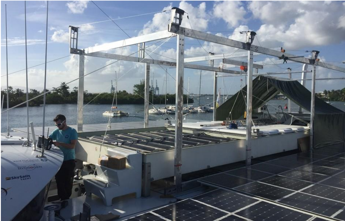
Figure 35: Compactable structure to protect the H 2 system from bad weather, fitted with a hoist for heavy load
