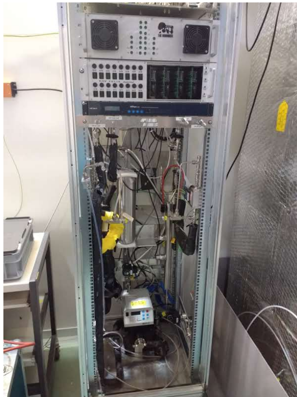
Figure 1 – The mobile electrolysis test bench realized in the frame of this project.
