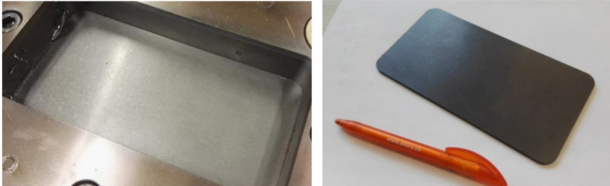
Figure 11: Plate in the mould after pressing (left) and demoulded plate (right)
