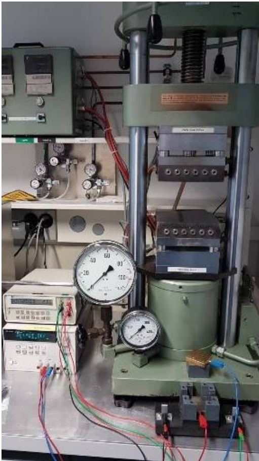
Figure 13: Through-thickness resistance measurements at PSI (left) and detail of the electrodes and the voltage wires (right).
