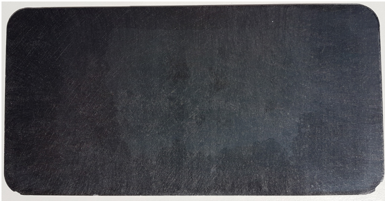
Figure 7: Plate composed of 50% EP, 45% Gr and 5% CB.
