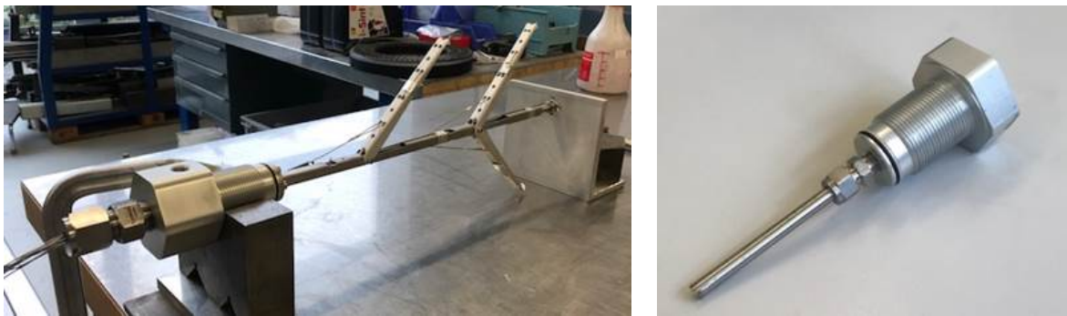
Figure 5 (Left) in-house developed thermocouple tree, (right) injection nozzle
