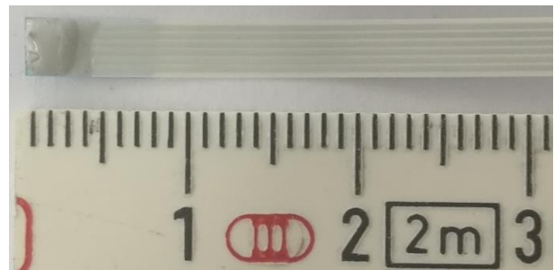
Figure 5-8: Pt100 temperature sensor covered with thermal conductive adhesive
