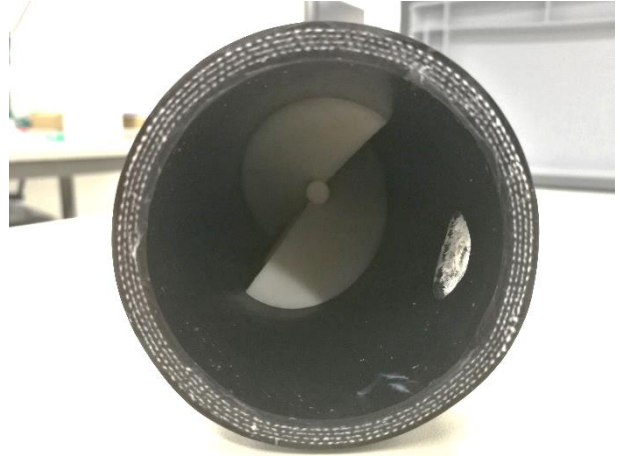
Figure 7-10: Static mixer inserted in the silicone hose
