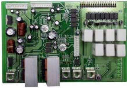
Bild 23: Batterie-Management System (BMS)
