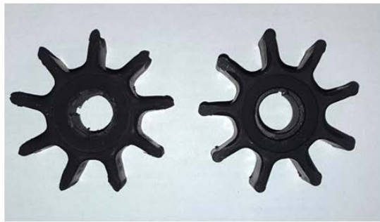
Figure 40: Comparison between a used FKM impeller (left) and a new FKM impeller (right). The impeller on the left shows clear signs of abrasion.
