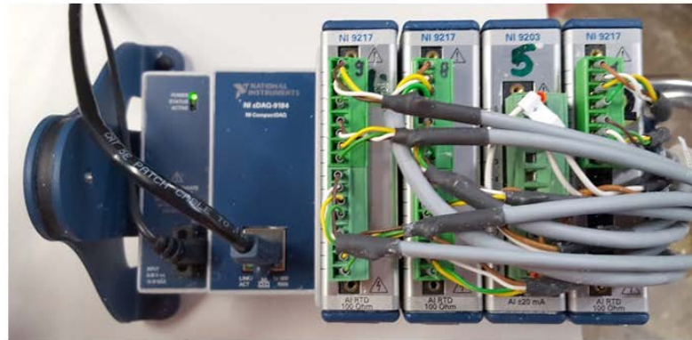
Figure 47: Photograph of the used chassis cDAQ-9184 of National Instruments with all connected wires.
