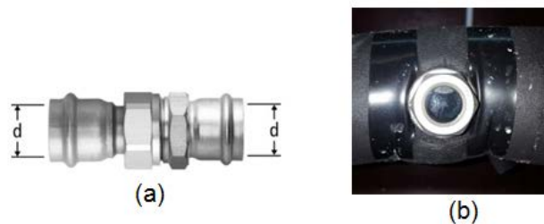
Figure 36: (a) Photograph of a press fitting used for the piping of the system. (b) Photograph of a viewing window which is used for an optical inspection of the flowing slurry.
