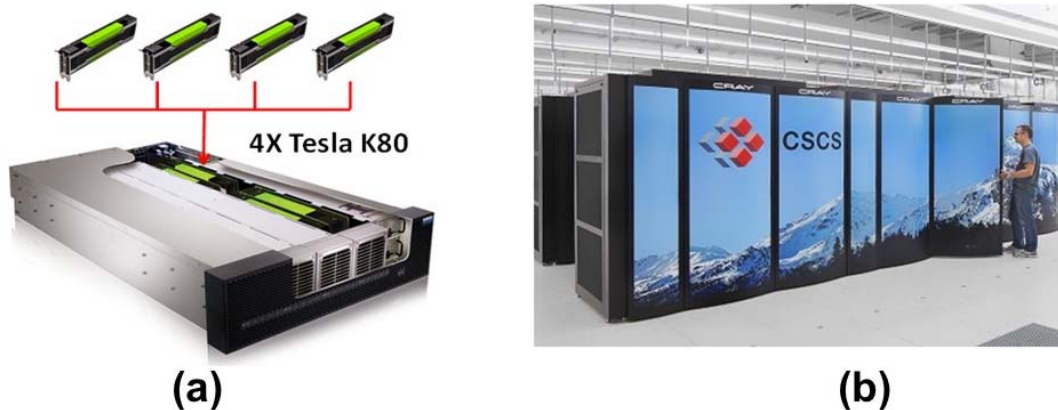
Fig. 20. (a) The local compute cluster of Dr. Mantzaras' group at PSI consisting of 4 Nvidia's Tesla K80 GPGPUs. (b) the Piz-Daint GPGPU cluster of the Swiss Supercomputing Center used for the long production runs
