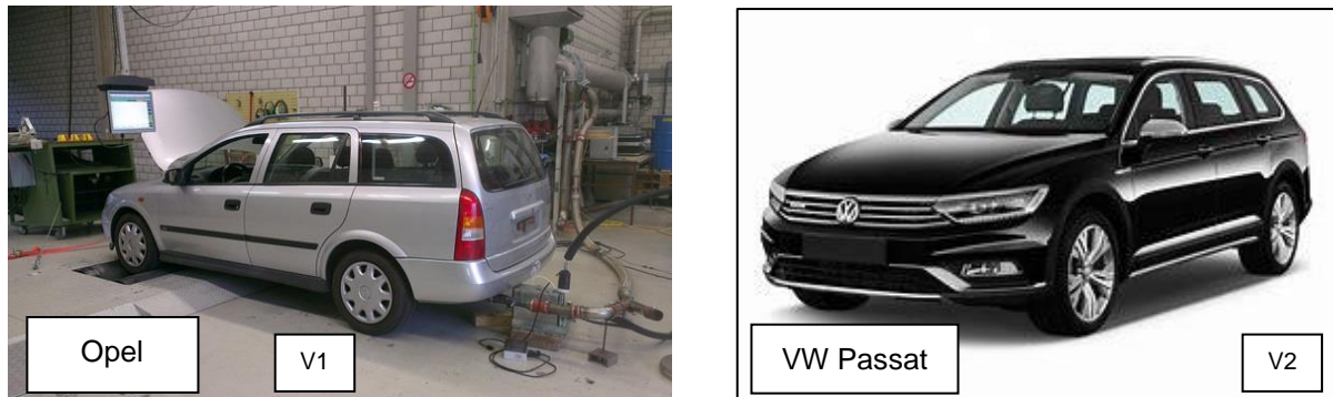
Fig. 20: Test vehicles Opel Astra (Euro 2) and VW Passat (Euro 6c) on chassis dynamometer
