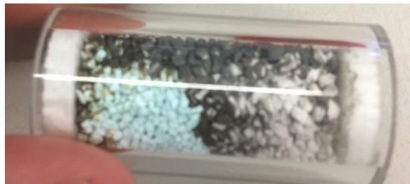
Figure 24. Demonstration of the color change of the total sulphur indicator SulfaTrack caused by sulphur in biogas in COSYMA.
