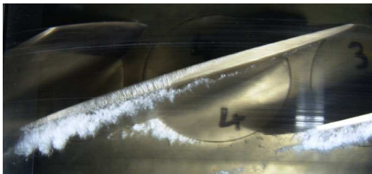
Axial blade – cavitation for H > 30 \text{ m}
