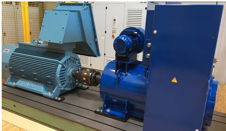
Figure 3: 0.5MW, 6kV rated Induction and Synchronous machines. ABB medium voltage drive ACS 2000 is visible behind.
