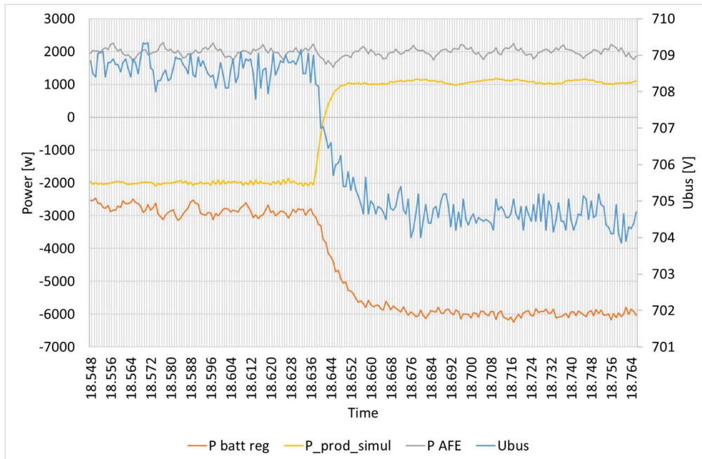
Figure 38: Zoom on the first event shown in Figure 37. It shows the power regulation of the regulation batteries and the AFE in response to a sudden positive power variation on the DC Link ( P_{prod\_simul} ). The time scale is in seconds, i.e. the time resolution reaches milliseconds in this measured trace by an oscilloscope.
