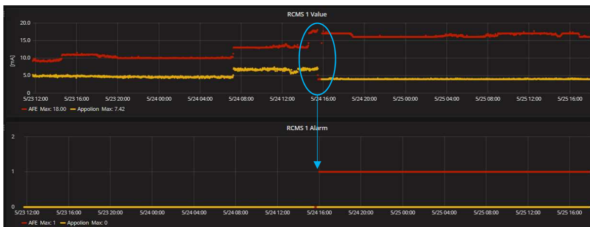
Figure 60: Leakage current measurements on the AFE (red) and on a storage battery pack (yellow).
