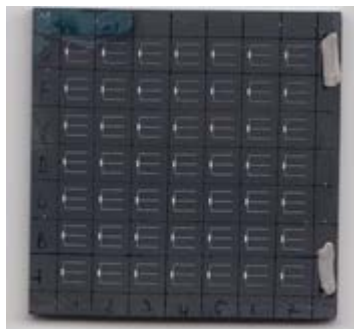
Fig. 2: Picture of a 5x5 cm 2 sample. Individual cells are 36 mm 2 .
