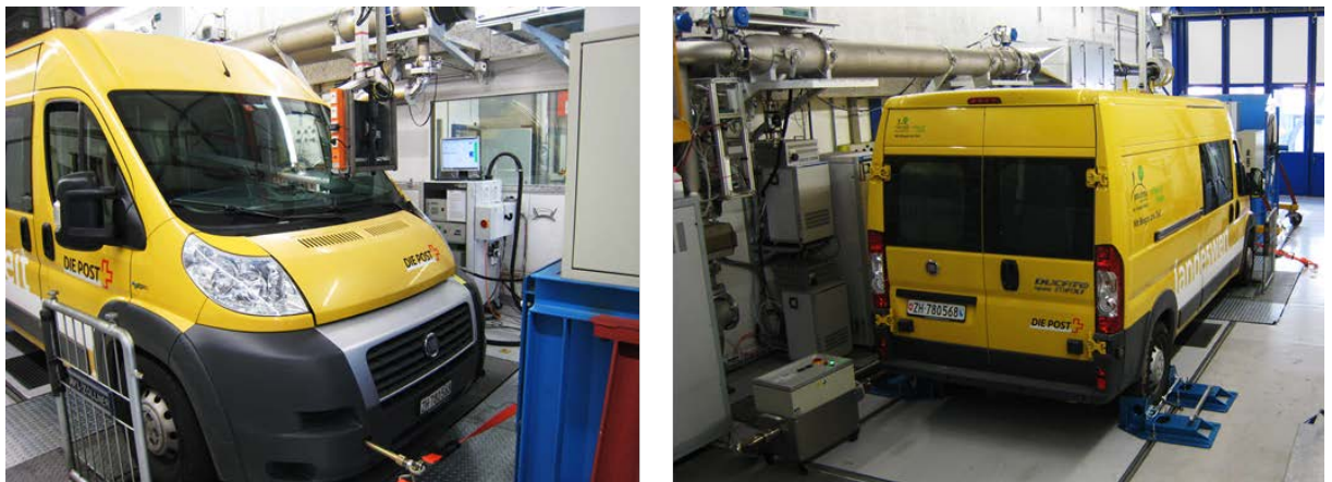
Fig. 34 Fiat Ducato from the Mobility Solution AG on the chassis dyno at Empa
