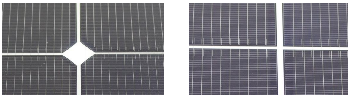
Figure 2.16: on left, picture of a regular SWCT module based on PSQ cells, the white diamond shape between cells produces no power. On right, rectangular shape cells leave minimal area between the cells, high cell density in module.
