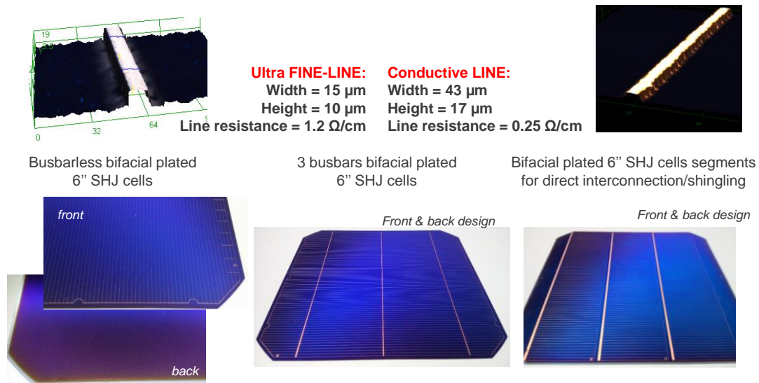
Figure 2.11: Pictures of full wafer 6" silicon heterojunction cells with the different plated metallization grid patterns defined, respectively for busbarless bifacial cells, 3 busbars bifacial cells and bifacial cells with specific design for cell segmentation followed by direct interconnection ("shingling").
