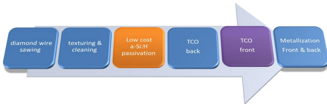
Figure 1.9: process flow of Si-HJT Gen 2 cells
