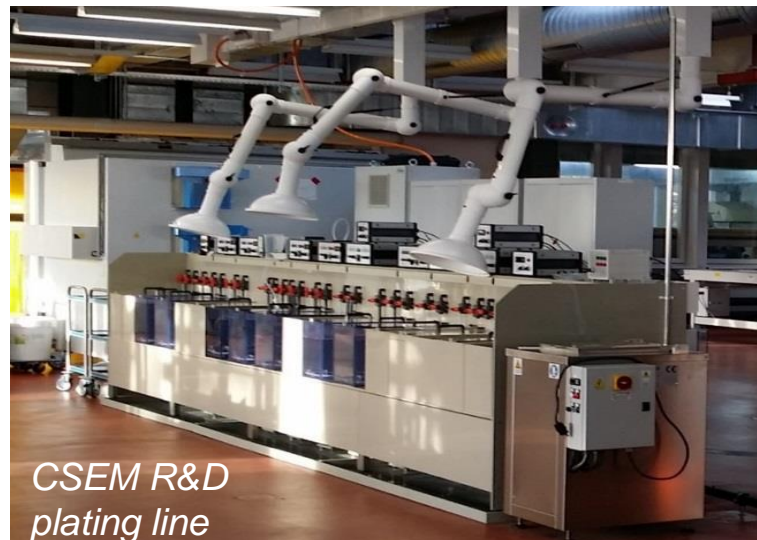
Figure 2.9: Picture of the CSEM R&D pilot line for plated metallization.
