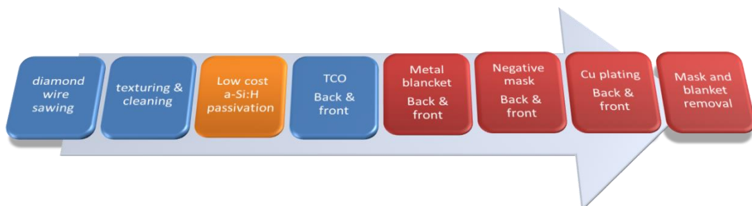
Figure 1.14: process flow of Si-HJT Gen 3.3 plated cells
