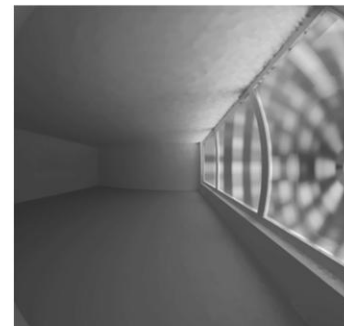
Figure 7: Daylight distribution for the Laser cut panel rendered with RADIANCE
