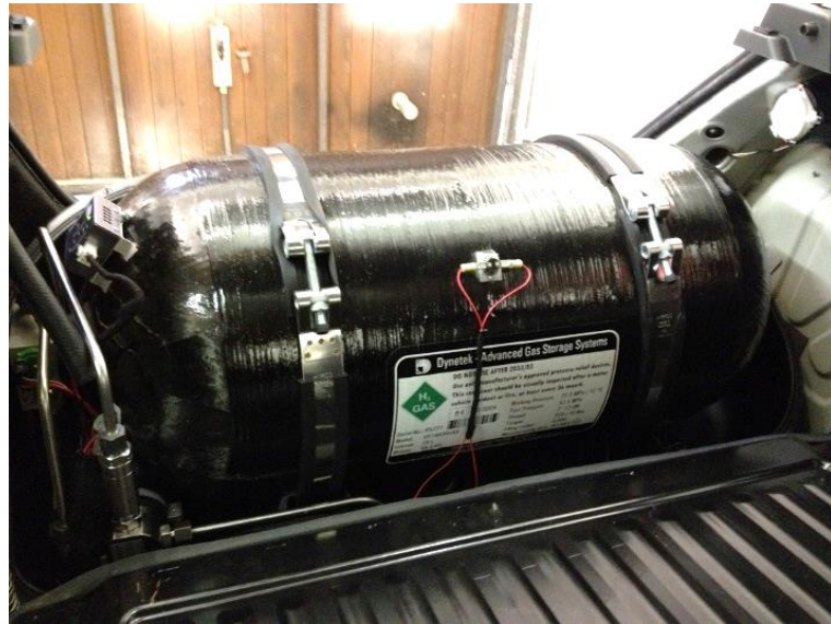
Fig. 11: Fixation system of the hydrogen tank.
