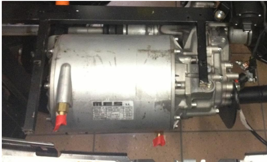
Fig. 15: The 21kW nominal power (60kW peak) electric motor supplied by MES.
