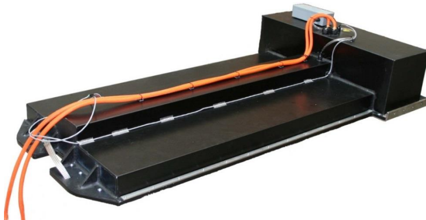
Fig. 13: The battery supplied by the Ökozentrum Langenbruck BL.
