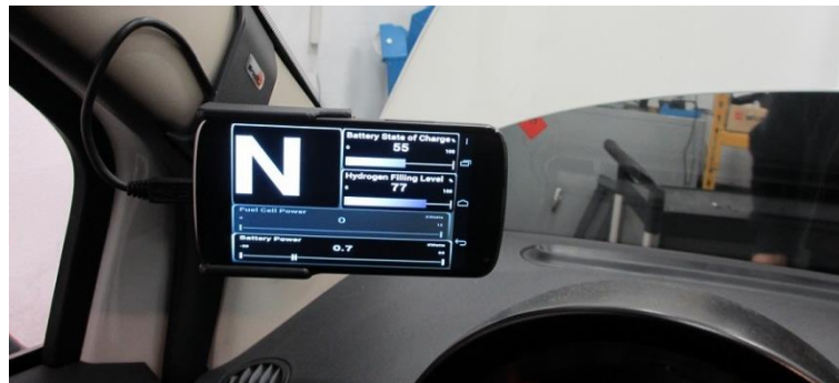
Fig. 20: Special display to give essential information's to the driver.
