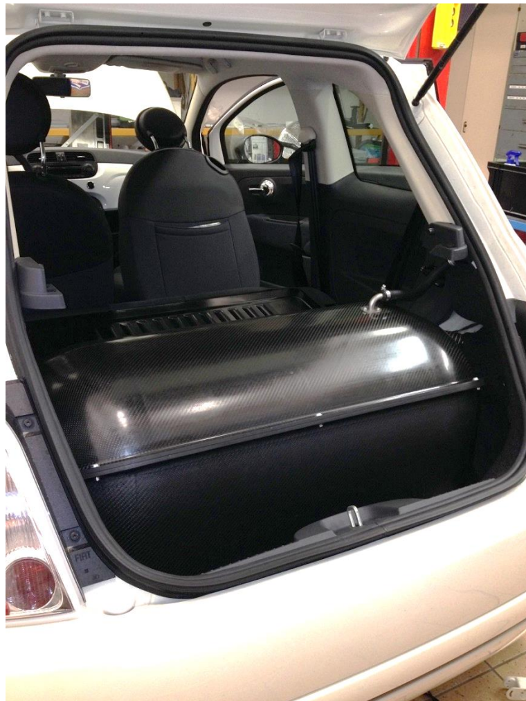
Fig. 12: Carbon fibre gas tight housing covering the hydrogen tank and its connections.
