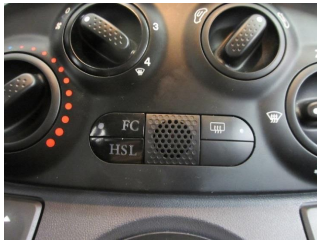
Fig. 19: User interface using unassigned buttons available in the Fiat 500.
