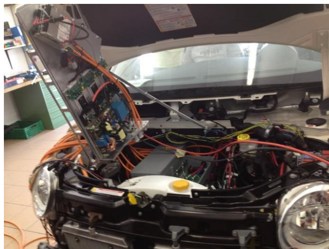
Fig. 18: The DC/DC-converter swung up with the different electronic modules mounted on its back cooling plate. There is a waterproof cover mounted over the back of the DC/DC during use.
