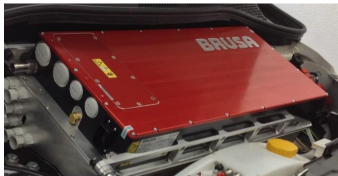
Fig. 17: The 110 kW DC/DC-converter supplied by Brusa.
