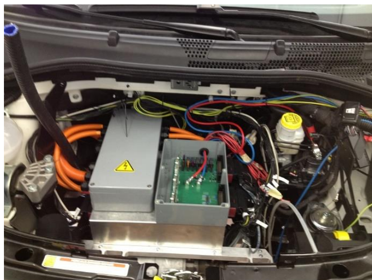
Fig. 21: Junction boxes. The box on the left is for the high voltage connections and fuses. The box on the right is for the low voltage connections.
