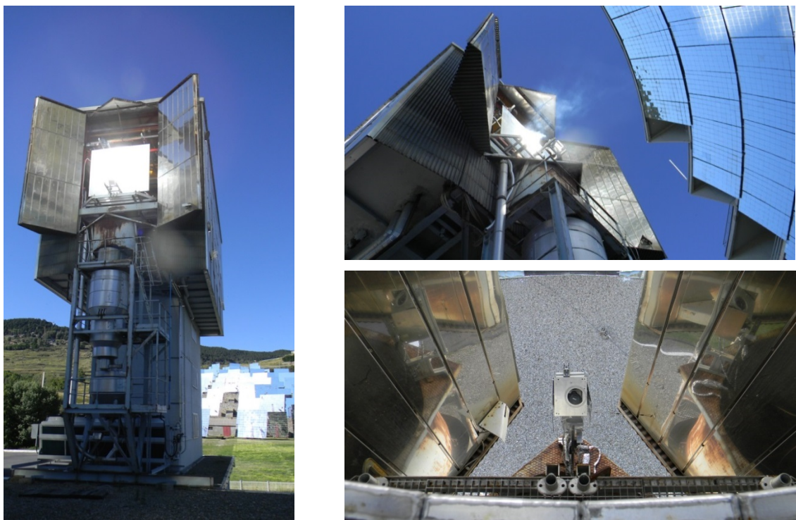
Figure 12: Operation of the solar reactor behind the spillage radiation shield on the MWSF tower (left) and visual camera mounted outside the spillage radiation shield on the experimental platform (right).
