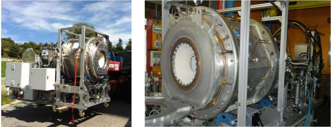
Figure 11: Solar reactor being moved into the MWSF tower (left) and mounted on experimental platform (right).
