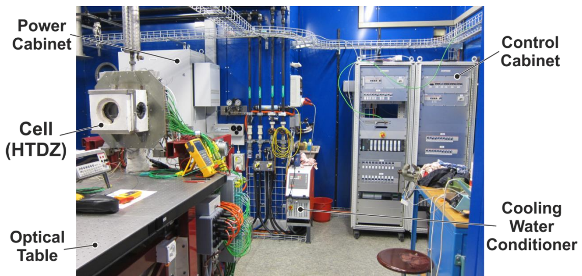
Figure 34: A view of the new HTDZ lab facility with the new control system
