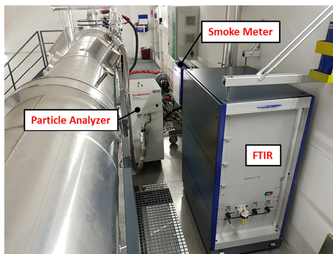
Figure 2 Exhaust gas analytics and soot measurement setup
