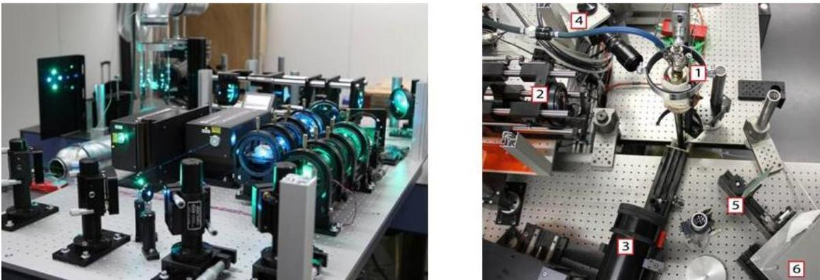
Figure 4: Left - Overview of PDA System. Right - Top view on the experimental setup with: (1) mono-disperse droplet generator, (2) front lens PDA transmitting optics, (3) PDA receiver
